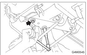
5) Remove bolts securing crossmember to car body, and remove crossmember.
