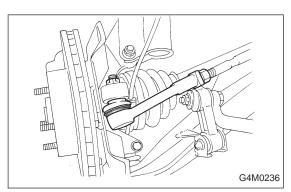
9) While depressing brake pedal, tighten axle nut and lock it securely.
