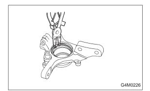
5) Using ST1 and ST2, press a new bearing into place.
