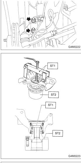
14) After scribing an alignment mark on camber adjusting bolt head, remove bolts which connect housing and strut, and disconnect housing from strut.
