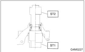
6) Using ST1, support housing securely.
