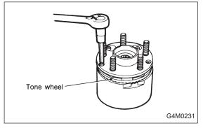
3) Remove foreign particles (dust, rust, etc.) from mating surfaces of hub and tone wheel, and install tone wheel to hub (only vehicle equipped with A.B.S.).
