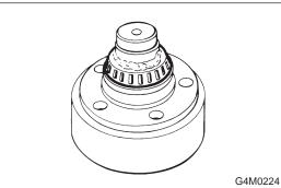
If inner bearing race remains in the hub, remove it with a suitable tool (commercially available).
