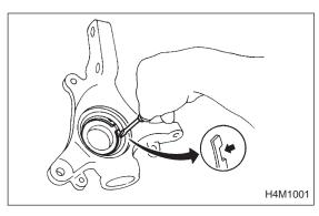
5) Using flat bladed screwdriver, remove snap ring.
