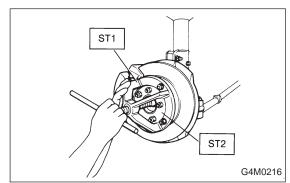
6) Remove DOJ from transmission spindle.
