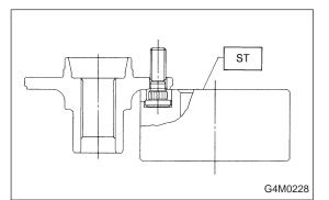
9) Using ST and a hydraulic press, drive hub bolts out.ST 927080000 HUB STAND
