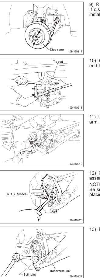
9) Remove disc rotor from hub.
