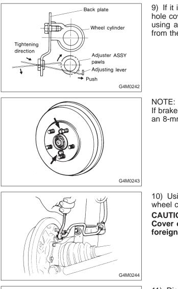
9) If it is difficult to remove brake drum, remove adjusting hole cover from back plate, and then turn adjusting screw using a slot-type screwdriver until brake shoe separates from the drum.
