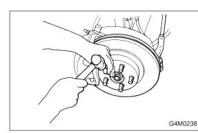
10) After tightening axle nut, lock it securely.
