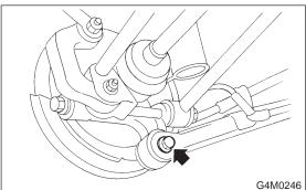
4) Connect rear housing assembly to trailing link assembly.
