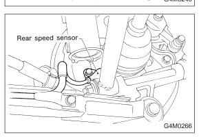
8) Install rear speed sensor to back plate (only vehicle equipped with A.B.S.).
