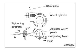
11) If it is difficult to remove brake drum, remove adjusting hole cover from back plate, and then turn adjusting screw using a slot-type screwdriver until brake shoe separates from the drum.
