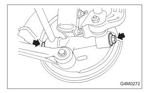
2) Connect rear spindle assembly to lateral link assembly.
