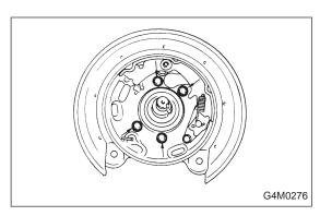
2) Remove back plate from rear spindle.
