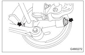
15) Remove bolts which secure lateral link assembly to rear spindle.
