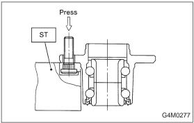
3) Using ST, press hub bolts out.
