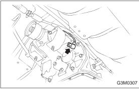
(3) Install vehicle speed sensor 1.
