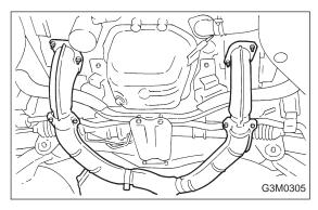
(3) Remove front exhaust pipe. Disconnect oxygen sensor connector, and remove exhaust pipe.
