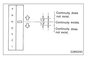
(4) Check if there is continuity at equal points when the select lever is turned 1.5° in both directions from the N range.
