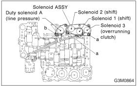
(7) Remove shift solenoids 1, 2, and 3, and duty solenoid A.
