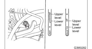
(10) Replenish ATF and check oil level. Check for leaks.
