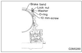
3) With the adjusting screw immobilized, tighten the lock nut.
