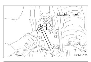
(5) Install propeller shaft.
