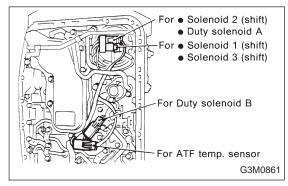
(5) Connect harness connectors at 4 places. Connect connectors of same color, and secure connectors to valve body using clips.
