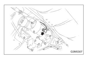
(6) Remove vehicle speed sensor 1.
