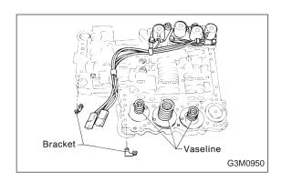
(3) Install valve body and two brackets.
