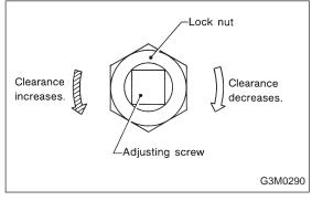
2) In case of the occurrence of problems 1 and 4 mentioned previously, perform the adjustment as follows: Adjusting procedure: Tighten adjust screw to 9 N·m (0.9 kg-m, 6.5 ft-lb) torque, then back off three turns.
