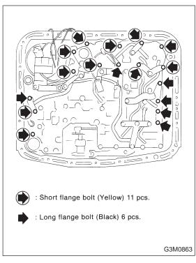
(6) Remove control valve body and two brackets. Remove 6 long bolts (Black) and 11 short bolts (Yellow).
