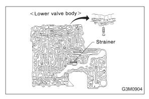
3) Install the orifice check valve, orifice check spring and filter to the lower valve body.
