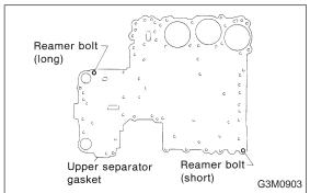
2) From under upper valve body, install two bolts using washers and position upper separator gasket.
