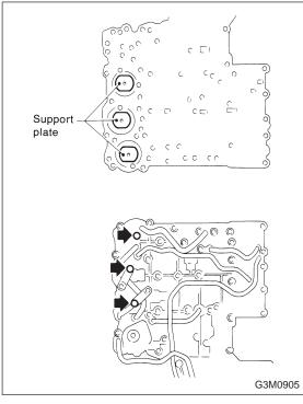
4) Install lower separate gasket and separate plate on lower body in that order, then temporarily tighten three support plates and two brackets.
