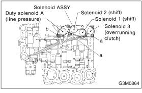
8) Install the shift solenoid and duty solenoid A.
