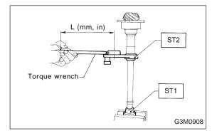
4) Tighten the lock washer and lock nut with ST1.
