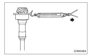
5) Measure the starting torque of the bearing. Make sure the starting torque is within the specified range.
