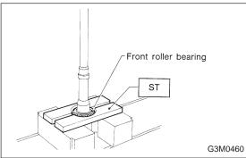
3) Using a press and ST, separate the front roller bearing from the shaft.
