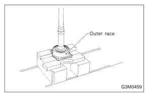
2) Using a press, separate the rear roller bearing and outer race from the shaft.
