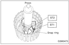
2) Set the retainer on the piston with a press using ST1 and ST2, and attach the snap ring.
