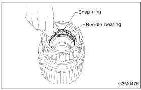
8) Remove the needle bearing after taking out the snap ring.
