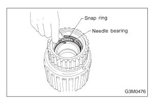
8) Install the needle bearing, and secure with the snap ring.
