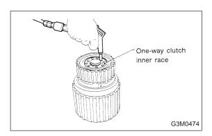
6) Check the forward clutch and overrunning clutch for operation.
