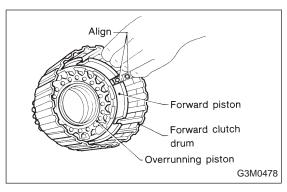
1) Fit the forward piston and overrunning piston to the forward clutch drum.
