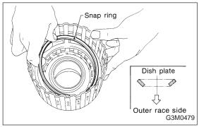
3) Install the dish plate, driven plates, drive plates, and retaining plate, and secure with the snap ring. (Overrunning clutch)
