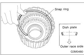
4) Install the dish plates, driven plates (1800 cc / 4 sheets, 2200 cc / 6 sheets), drive plates (1800 cc / 4 sheets, 2200 cc / 6 sheets), and retaining plate, and secure with the snap ring. (Forward clutch)
