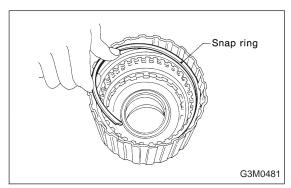
5) Install the snap ring (for front planetary carrier).
