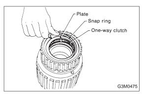
7) Remove the one-way clutch after taking out the snap ring.
