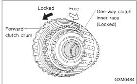
8) Install the one-way clutch (1-2) and plate, and secure with the snap ring.
