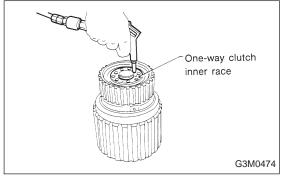
6) Install the one-way clutch inner race to the forward clutch drum, and apply compressed air to remove the over-running piston and forward piston.
