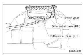
2) Install the washer and differential bevel gear to the differential case (LH). Then put the case over the differential case (RH), and connect both cases.
