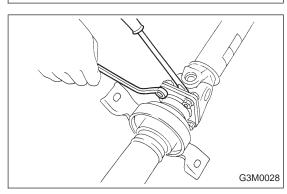
2) Remove bolts which hold front propeller shaft to rear propeller shaft.
