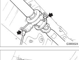
10) Remove propeller shaft from transmission.
