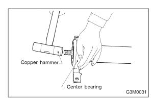
5) Lightly tap the head of front propeller shaft with a copper hammer until center bearing is removed.
