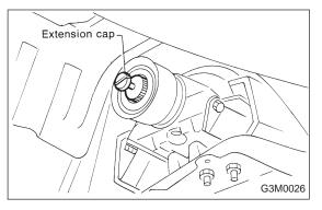
11) Install the extension cap to transmission.
