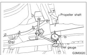
3) Runout of propeller shaft
