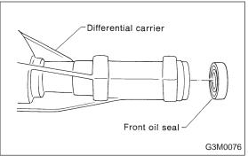
19) Remove front oil seal from differential carrier using ST. 398527700 PULLER ASSY
