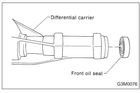
18) Remove front oil seal from differential carrier.
