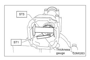
(2) Measure the clearance N between the end of ST3 and the end surface of ST1 by using a thickness gauge.
