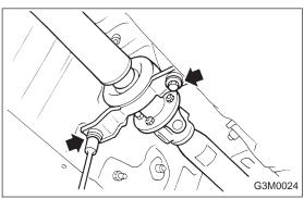
10) Remove propeller shaft.
