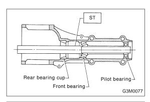
19) Remove pilot bearing together with front bearing cone using ST.
