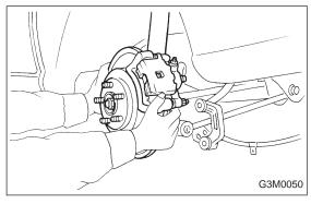
(4) Completely insert DOJ into rear differential by pressing rear housing.
