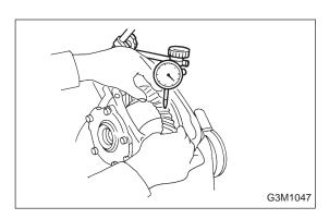
15) Re-check crown gear-to-pinion backlash.
