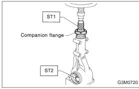
9) Press-fit companion flange with ST1 and ST2 until shaft protrudes 10 to 15 mm (0.39 to 0.59 in) beyond flange.
