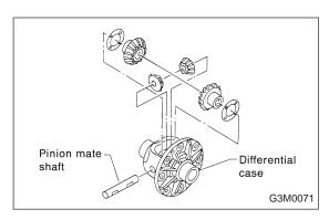
14) Draw out pinion mate shaft and remove pinion mate gears, side gears and thrust washers.
