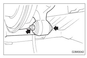
(5) Remove the bolts which secure the trailing link to the rear housing.
