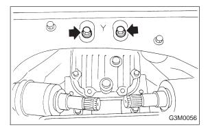
17) Remove self-locking nuts connecting rear differential to rear crossmember.
