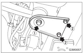
18) Remove bolts which secure rear differential front member to body.
