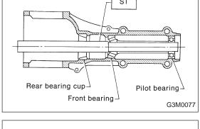
21) When replacing bearings, tap front bearing cup and rear bearing cup in this order out of case by using a brass bar.
