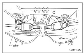
14) Secure rear drive shaft to rear crossmember using wire.
