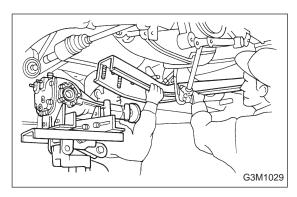
20) While slowly lowering transmission jack, move rear differential forward and remove front member and rear differential from body.
