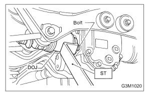
(7) Remove the DOJ from the rear differential by using ST.
