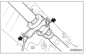
10) Remove propeller shaft.
