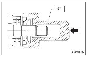
11) Fit a new oil seal using ST. ST 498447120 OIL SEAL INSTALLER
