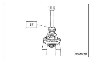
13) Press side bearing cone onto differential case with ST1.
