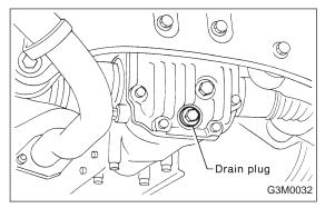
4) Remove oil drain plug, and drain gear oil.
