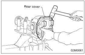
3) Remove rear cover by loosening retaining bolts.
