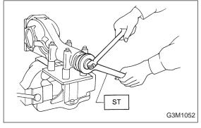
11) Hold companion flange with ST and remove drive pinion nut.
