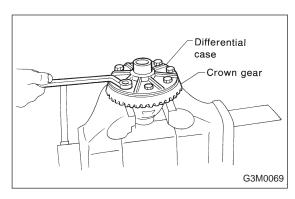
9) Remove crown gear by loosening crown gear bolts.
