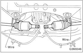
14) Secure rear drive shaft to rear crossmember using wire.
