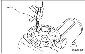
10) Drive out pinion shaft lock pin from crown gear side. NOTE:
