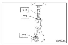
6) Press-fit front bearing cone into case with ST1, ST2 and ST3.
