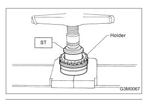
9) Remove oil seal from right and left holders with ST.
