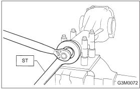
15) Hold companion flange with ST and remove drive pinion nut.
