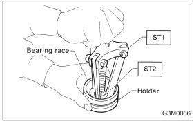
8) Remove bearing race from right and left holders with ST1 and ST2.
