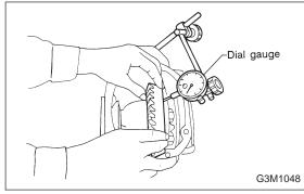
16) Check the crown gear runout on its back surface, and make sure pinion and crown gear rotate smoothly.
