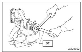
10) Install self-locking nut. Then tighten it with ST.
