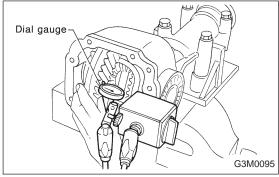
17) Re-check crown gear-to-pinion backlash.
