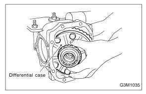
6) Pull out differential case assembly from differential carrier.
