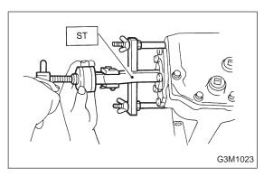
10) Remove side oil seal with ST.ST 398527700 PULLER ASSY
