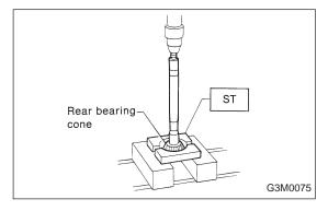
18) Remove rear bearing cone from drive pinion by supporting cone with ST.
