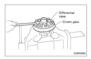
11) Install crown gear on differential case.
