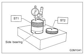
12) Before installing side bearing, measure the bearing width by using a dial gauge, ST1 and ST2.
