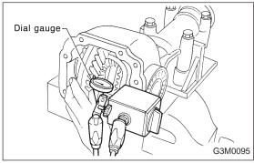
(6) Measure the crown gear-to-drive pinion backlash. Set magnet base on differential carrier. Align contact point of dial gauge with tooth face of crown gear, and move crown gear while holding drive pinion still. Read value indicated on dial gauge.
