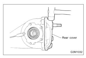
4) Remove rear cover by loosening retaining bolts.
