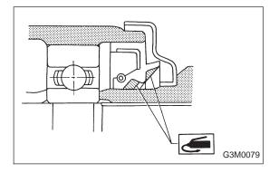
(7) Replace the oil seal with new one at every disassembly. Apply chassis grease between the lips when installing the oil seal.
