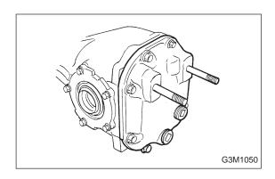
19) Install rear cover and tighten bolts to specified torque.
