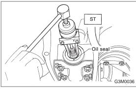
9) Remove oil seal using ST. ST 499705401 PULLER ASSY
