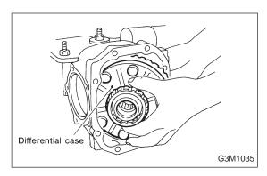
(3) Install the differential case assembly into differential carrier in the reverse order of disassembly.
