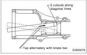
20) When replacing bearings, tap front bearing cup and rear bearing cup in this order out of case by using a brass bar.
