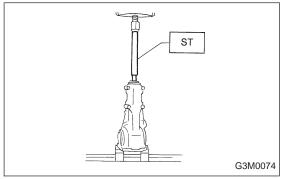
17) Press the end of drive pinion shaft and extract it together with rear bearing cone, preload adjusting spacer and washer.
