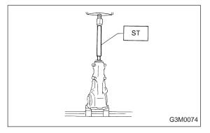
13) Press the end of drive pinion shaft and extract it together with rear bearing cone, preload adjusting spacer and washer.
