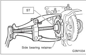
5) Make right and left side bearing retainers in order to identify them at reassembly. Remove side bearing retainer attaching bolts, set ST to differential case, and extract right and left side bearing retainers with a puller.
