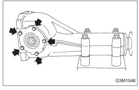
(5) Tighten side bearing retainer bolts.
