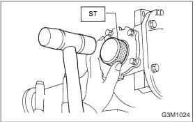
11) Drive in a new side oil seal with ST.
