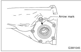
(4) Fit the selected shims and O-ring on side bearing retainer and install them on differential carrier with the arrow mark on the retainer directed as shown in figure.
