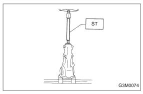
16) Press the end of drive pinion shaft and extract it together with rear bearing cone, preload adjusting spacer and washer.
