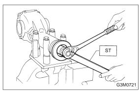
10) Install self-locking nut. Then tighten self-locking nut with ST.
