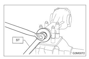
14) Hold companion flange with ST and remove drive pinion nut.
