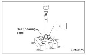
17) Remove rear bearing cone from drive pinion by supporting cone with ST.
