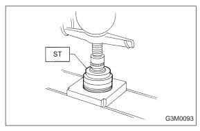
(2) Install bearing race into right and left holders.ST 398477702 BEARING OUTER RACE DRIFT
