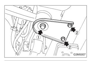
18) Remove bolts which secure rear differential front member to body.
