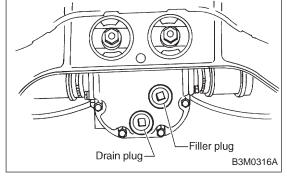
4) Remove oil drain plug, and drain gear oil.
