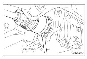
13) Remove DOJ of rear drive shaft from rear differential. <Ref. to 3-4 [W2A2].>
