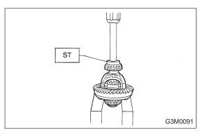
12) Press side bearing cone onto differential case with ST. ST 498485400 DRIFT
