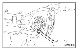
(5) Temporarily tighten lock plate.
