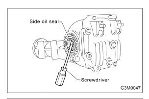
10) Remove oil seal with screwdriver.
