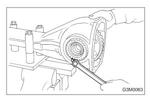
16) Tighten bolt of lock plate to specified torque.
