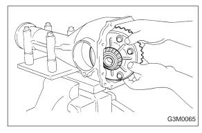
7) Pull out differential assembly from differential carrier.
