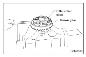
12) Drive out pinion shaft lock pin from crown gear side. NOTE:
