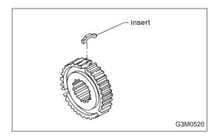
5) Insert (shifting) Replace the insert if deformed, excessively worn, or defective in any way.
