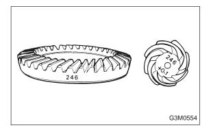
1) Alignment marks/figures on hypoid gear set ① The upper figure on driven pinion is the match number for combining it with hypoid driven gear. The lower figure is for shim adjustment. If no lower figure is shown, the value is zero. The figure on hypoid driven gear indicates a number for combination with drive pinion.
