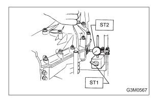
(8) Set ST1 and ST2. Insert the needle through transmission oil drain plug hole so that the needle comes in contact with the tooth surface at a right angle and check the backlash.
