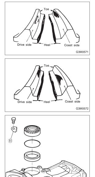
• The drive pinion shim selected before is too thick. Reduce its thickness.
