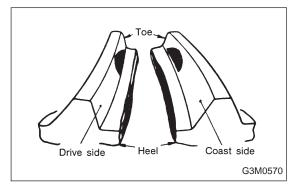
(9) Check tooth contact of hypoid gear as follows: Apply a uniform thin coat of red lead on both tooth surfaces of 3 or 4 teeth of the hypoid gear. Move the hypoid gear back and forth by turning the transmission main shaft until a definite contact pattern is developed on hypoid gear, and judge whether face contact is correct. If it is incorrect, make the following correction.
