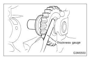
(2) After installing a suitable reverse shifter lever, shift into Neutral. Adjust clearance between reverse idler gear and transmission case wall, using washer(s).
