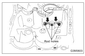
1) Position interlock plungers (5.56 x 19.6), one plunger in hole between 1-2 and 3-4 fork rod holes, and one plunger in hole between 3-4 and reverse fork rod holes.
