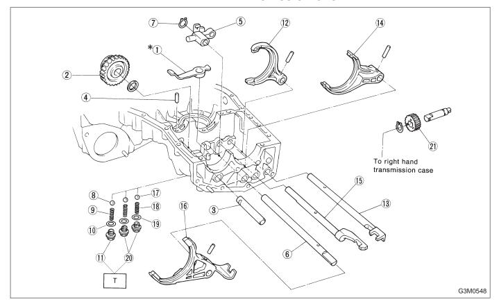
Tightening torque: N·m (kg-m, ft-lb) T: 18.1 — 21.1 (1.85 — 2.15, 13.4 — 15.6)
