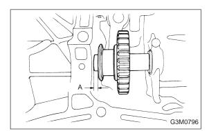
5) Adjustment of reverse idler gear position.
