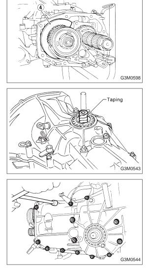
3) Remove main shaft rear plate ④.
