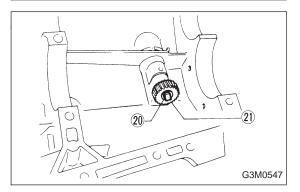
9) Remove outer snap ring (2) and pull out speedometer driven gear (21). Next, remove speedometer shaft (22) and washer.
