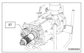
10) Backlash adjustment of hypoid gear and preload adjustment of roller bearing.
