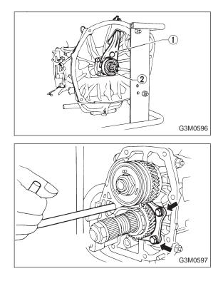
1) Remove clutch release lever (1) and bearing (2). <Ref. to 2-10 [W3A0].>
