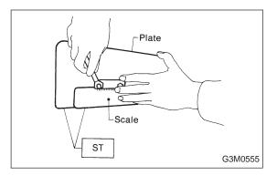
2) Adjustment of drive pinion shim (2)
