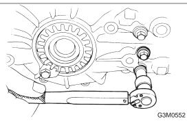
9) Position balls (7.1438 mm dia.) (17), checking ball springs (18) and gaskets (19) into 3-4 and 1-2 rod holes, and install plugs (20).
