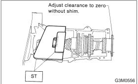
(3) Position the ST by inserting the knock pin of ST into the knock hole in the transmission case.
