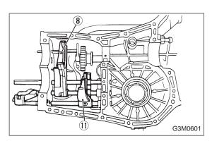
3) Drive out straight pin (6), and pull out 3-4 fork rod (7) and shifter fork (8).
