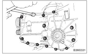
(2) Separate transmission case into right and left cases by loosening seventeen coupling bolts and nuts.
