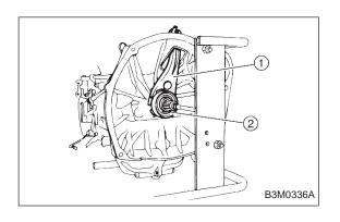
13) Install clutch release lever ① and bearing ②. <Ref. to 2-10 [W3C0].>
