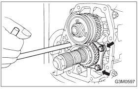
2) Remove bearing mounting bolts.
