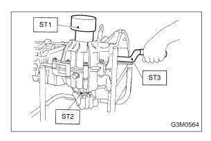
(1) Place the transmission with case left side facing downward and put ST1 on bearing cup.
