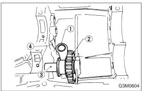
2) Install reverse shifter lever ①, reverse idler gear ② and reverse idler gear shaft ③, and secure with straight pin ④. NOTE:
