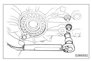
9) Position balls ①, checking ball springs ⓐ and gaskets ① into 3-4 and 1-2 rod holes, and install plugs ②.
