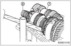
5) Remove drive pinion shaft assembly 6 from left side transmission case.
