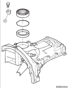
(4) Fit lock plate ①. Loosen the retainer on the lower side by 1-1/2 notches of lock plate and turn in the retainer on the upper side by the same amount in order to obtain the backlash.
