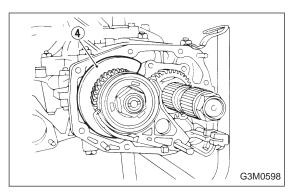
3) Remove main shaft rear plate 4).
