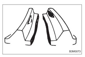
• The drive pinion shim selected before is too thick. Reduce its thickness.
