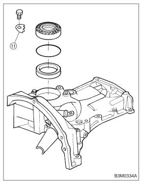
11) After checking the tooth contact of hypoid gears, remove the lock plate ①. Then loosen retainer until the O-ring groove appears. Fit O-ring into the groove and tighten retainer into the position where retainer has been tightened in.
