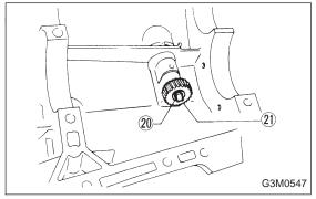
9) Remove outer snap ring (20) and pull out speedometer driven gear (1). Next, remove oil seal, speedometer shaft (2) and washer.
