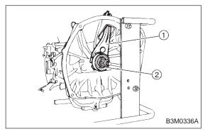
1) Remove clutch release lever 1 and bearing 2. <Ref. to 2-10 [W3A0].>
