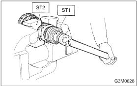
11) Install lock washer and tighten lock nut to the specified torque using ST1 and ST2.
