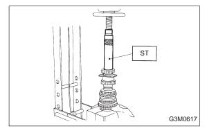
10) Position woodruff key in groove on the rear of drive pinion shaft. Install 5th driven gear onto drive shaft using ST and press.
