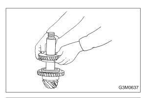
5) Install 1st driven gear, 1st-2nd balk ring and gear and hub assembly (already assembled in previous step) to drive pinion shaft by hand.
