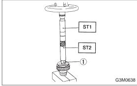
6) Install 1st-2nd driven gear bushing ① to drive pinion shaft using ST1 and ST2.
