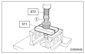
3) Install 4th needle bearing race (1) onto transmission main shaft using ST1, ST2 and a press.
