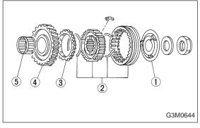
3) Remove insert stopper plate (1), sleeve and hub assembly No. 2, baulk ring (3), 5th drive gear (4), and needle bearing (5) (32 x 36 x 25.7).
