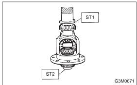
4) Install roller bearing (40 x 80 x 19.75) to differential case.
