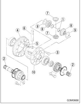
3) Align pinion shaft and differential case at their holes, and drive straight pin (5) into holes from the hypoid driven gear side, using ST.
