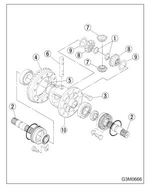
4) Pull out pinion shaft (6), and remove differential bevel pinion (7) and gear (8) and washer (9).
