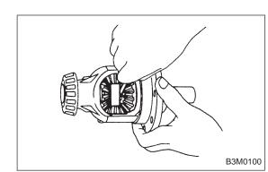
6) Position drive axle shaft in differential case and hold it with outer snap ring (28). Using a thickness gauge, measure clearance between the shaft and case is within specifications.
