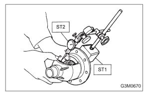
2) Measure backlash between bevel gear and pinion. If it is not within specifications, install a suitable washer to adjust it.
