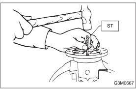
3) Drive out straight pin (5) from differential assembly toward hypoid driven gear.
