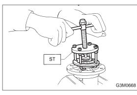
5) Remove roller bearing using ST. ST 399527700 PULLER SET
