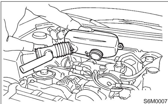
3) Remove air intake chamber stay. (AT vehicles only)
