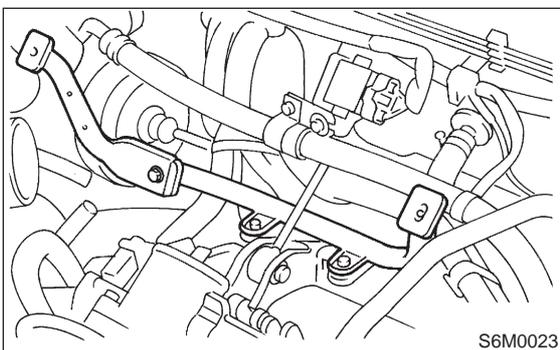
4) Disconnect connector and terminal from starter.
