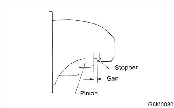
2) If motor is running with the pinion forced endwise on the shaft, disconnect connector from terminal M of switch assembly and connect terminal M to ground terminal (–) of battery with a lead wire. Next, gently push pinion back with your fingertips and measure pinion gap.
