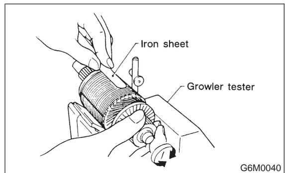
5) Armature ground test
