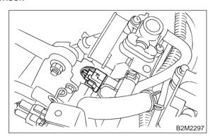
7) Disconnect air by-pass hose from idle air control solenoid valve.
