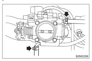
9) Remove bolts which install throttle body to intake manifold.
