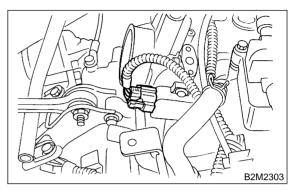
8) Disconnect connector from idle air control solenoid valve.
