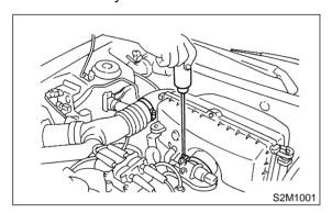
4) Disconnect blow-by hose and air hoses, and remove air intake chamber.
