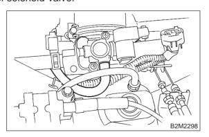
8) Disconnect engine coolant hoses from throttle body.
