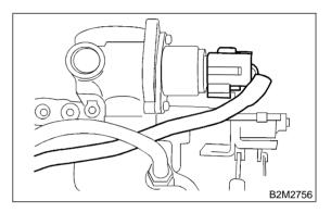
9) Disconnect engine coolant hoses from throttle body.
