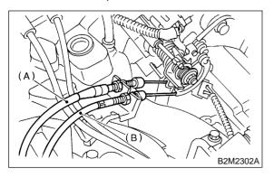
7) Disconnect connector from throttle position sensor.
