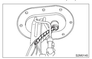
10) Remove bolt which installs fuel meter unit on mounting bracket.
