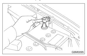
4) Disconnect connector from fuel pump.
