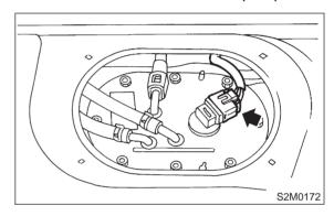
6) Disconnect quick connector, and then disconnect fuel delivery hose (A). <Ref. to 2-8 [W7A0].> 7) Move clips, and then disconnect fuel return hose (B) and jet pump hose (C).
