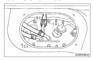
8) Remove nuts which install fuel pump assembly onto fuel tank.
