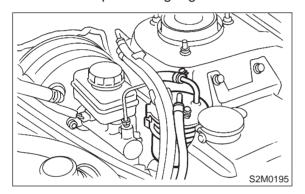
4) Connect connector to fuel pump relay.
