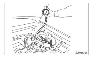
7) After connecting pressure regulator vacuum hose, measure fuel pressure.
