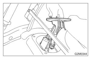
10) Drain fuel from fuel tank by using a hand pump.
