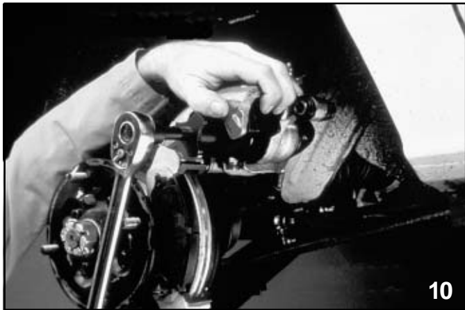
Depressing caliper piston (older)
