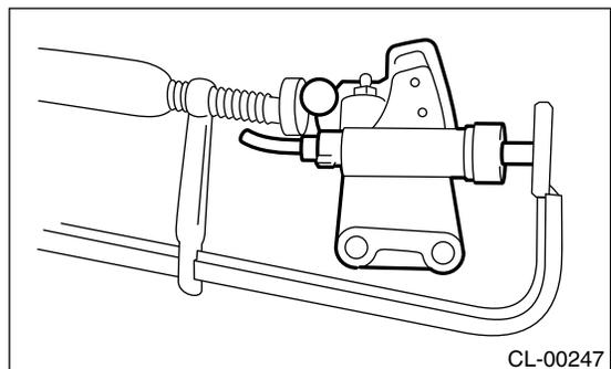
3) Fit one end of a vinyl tube into the air bleeder of operating cylinder and put the other end into a brake fluid container.
