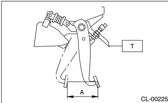
2) Turn the master cylinder push rod so that clevis pin moves to the left and then to the right. Clevis pin must move without resistance while it is rattling.
