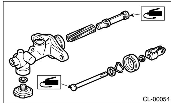
3) To assemble the master cylinder, reverse the sequence of disassembly procedure.
