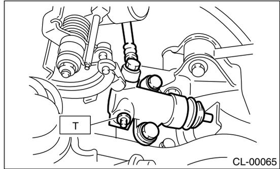
6) After depressing the clutch pedal, make sure that there are no leaks evident in the entire system.
