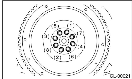
3) Install the clutch disc and cover. <Ref. to CL-11, INSTALLATION, Clutch Disc and Cover.>
