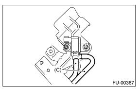
6) Remove the wastegate control solenoid valve from bracket.
