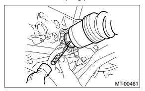
15) Install the ball joint of transverse link to housing.
