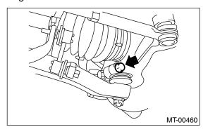
18) Using the ST, remove the spring pin of front drive shaft.
