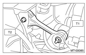
9) Install the clutch operating cylinder.
