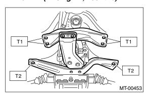
5) Lower the vehicle and install the fixing bolt.
