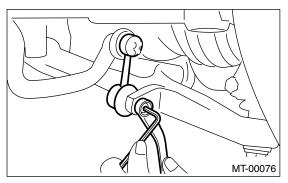
17) Remove the ball joint of transverse link from housing.
