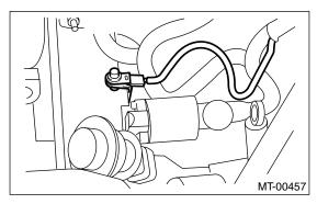
12) Connect the connector located on the upper side of transmission.
