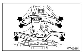
21) Move the transmission to right side, then remove the joint COMPL, stay bolt and reverse check cable.
