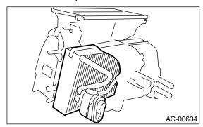
4) Loosen the two bolts to remove the expansion valve.
