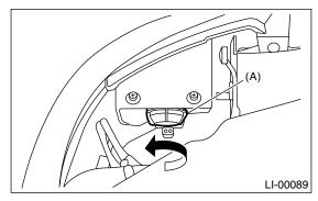
5) Remove the spring retainer, and then detach the fog light bulb.
