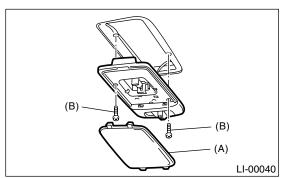
3) Disconnect the harness connectors and remove the light.
