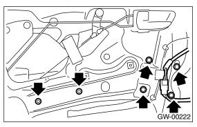
5) Loosen the screw to remove motor assembly.
