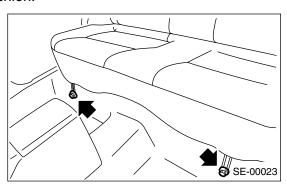
2) Remove the bolts securing lower portion of backrest and then open the center trunk through lid.
