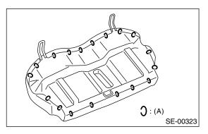
6) Remove the hog rings (A), and then remove the seat cover.
