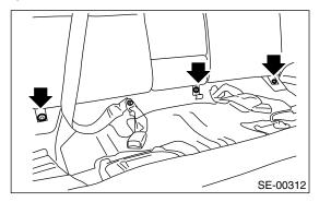
3) Hook and fasten the seat cushion to the hook on the lower part of the rear seat backrest.
