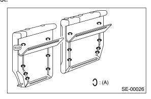
3) Remove the hog rings (A) on front side of cushion pad, and remove the cover.
