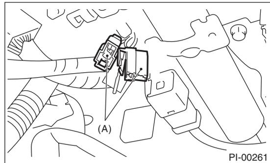
3) Connect the general scan tool to its data link connector in the lower portion of instrument panel (on the driver's side).
