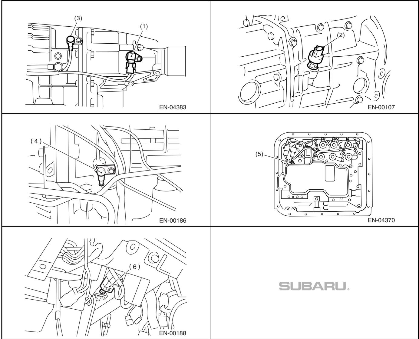
(1) Rear vehicle speed sensor (AT model)
