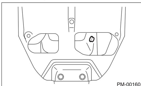
5) Using engine oil of proper quality and viscosity, fill engine oil through the oil filler duct to the upper level on level gauge. Place the vehicle on a level surface when checking oil level.
