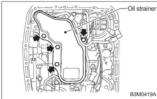
4) Install the oil strainer to the control valve. Be careful not to cut or break the O-ring. Then tighten four bolts.
