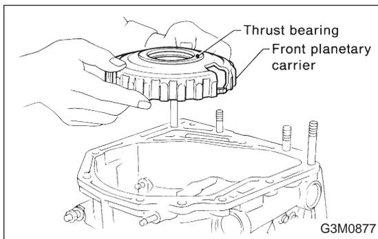
18) Take out the front planetary carrier and the thrust bearing.
