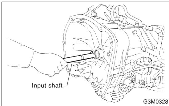
5) Remove the input shaft.
