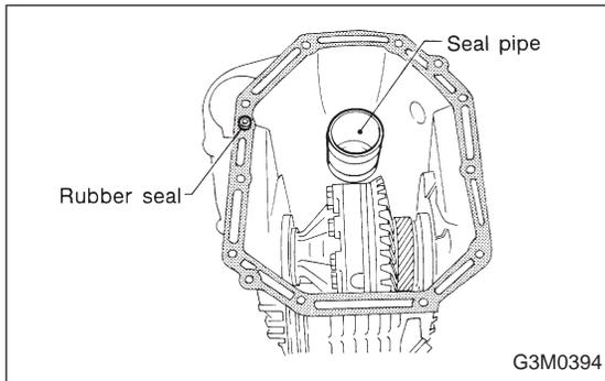
17) Install the rubber seal to the torque converter clutch case.
