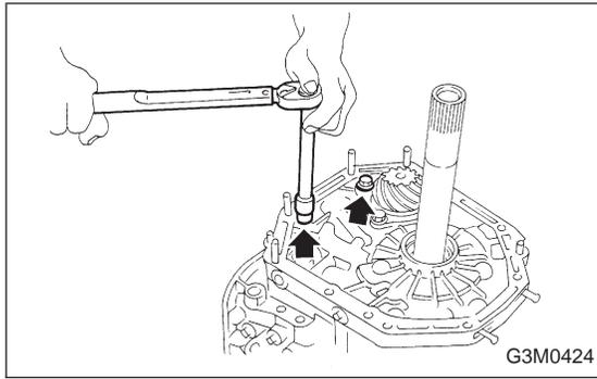
(4) Secure the housing with two nuts.
