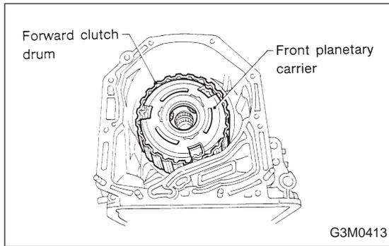
17) Install the front planetary carrier. Attach the thrust needle bearings to both sides of the carrier with vaseline. Install the carrier carefully, while aligning with the splines of the forward clutch drum, and while rotating the pinion.
