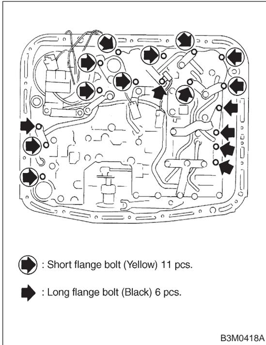
3) Install the control valve assembly.
