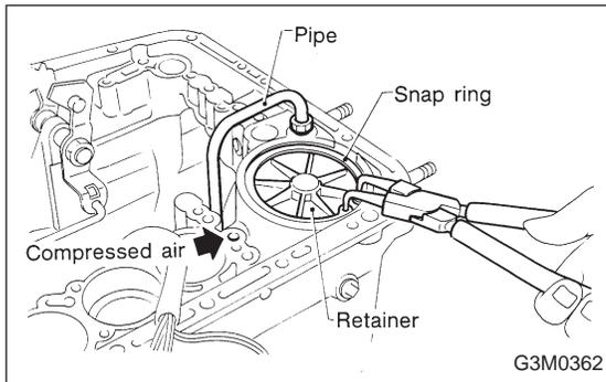
25) After removing the snap ring (inner), take out the servo piston by applying compressed air from the release pressure side.
