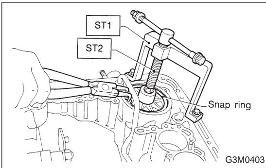
8) Install the band servo sub assembly.
