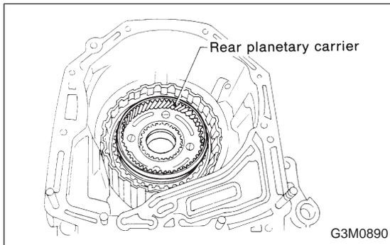
15) Install the rear planetary carrier.
