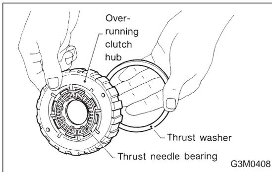
12) Assemble the overrunning clutch hub.
