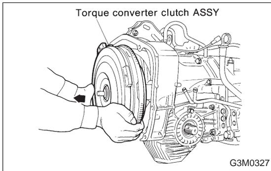
4) Extract the torque converter clutch assembly.
