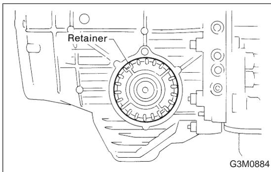
(5) Tighten the LH retainer until contact is felt while rotating the shaft. Then loosen the RH retainer. Keep tightening the LH retainer and loosening the RH retainer until the pinion shaft can no longer be turned. This is the "zero" state.
