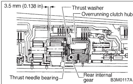
14) Assemble the rear internal gear.
