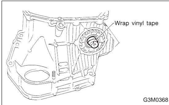
8) Wrap vinyl tape around the splined portion of the axle shaft.
