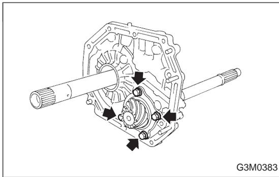
(2) Tighten four bolts to secure the roller bearing.
