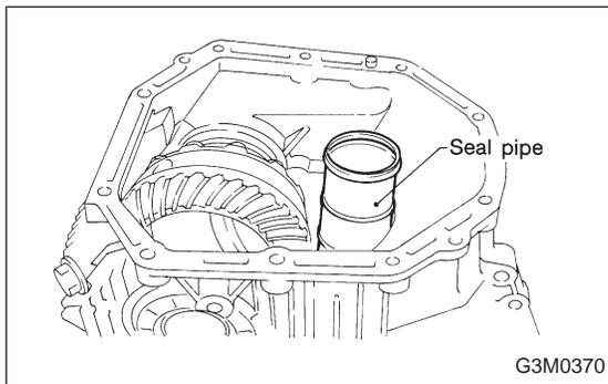
4) Remove the differential case assembly.
