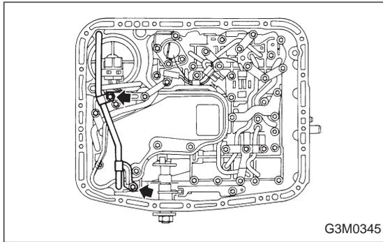
6) Install the oil cooler outlet pipe, and secure with two bolts.
