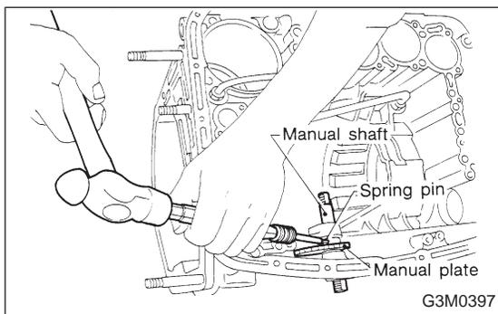
3) Install the manual plate and shaft, and secure with a spring pin.
