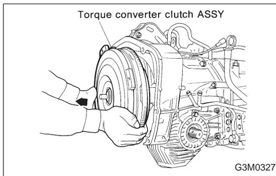
12) Install the torque converter clutch assembly.
