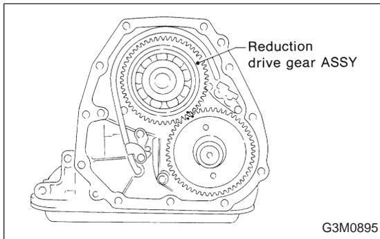
5) Install the reduction drive gear assembly.
