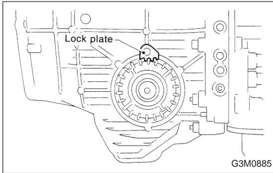
(9) If tooth contact is correct, mark the retainer position and loosen it. After fitting the O-ring, screw in the retainer to the marked position. Then tighten the lock plate to the specified torque.
