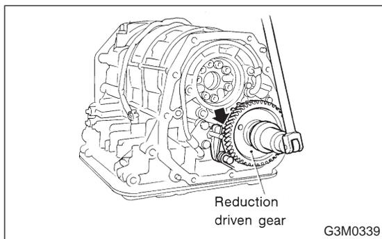
2) Remove the reduction driven gear.
