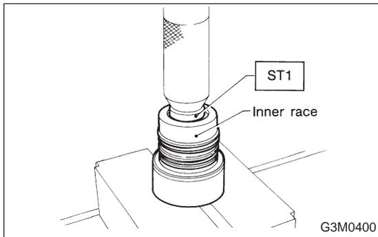
7) Install the one-way clutch inner race.
