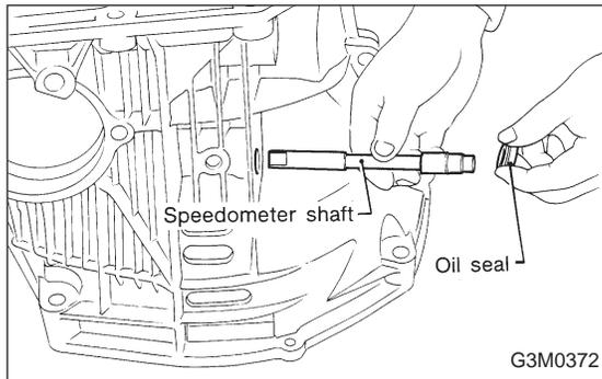
6) Remove vehicle speed sensor 2.
