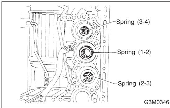
11) Remove the three accumulator springs.
