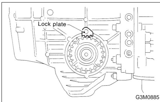
(6) After the "zero" state is established, back off the LH retainer 3 notches and secure it with the lock plate. Then back off the RH retainer and retighten until it stops. Repeat this procedure several times. Tighten the RH retainer 1-3/4 notches further. This sets the preload. Finally, secure the retainer with its lock plate.
