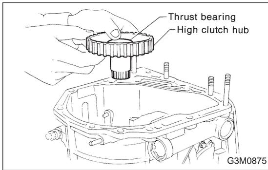
16) Take out the high clutch hub and the thrust bearing.
