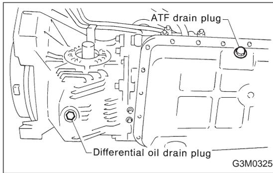
10) Tighten the drain plugs.
