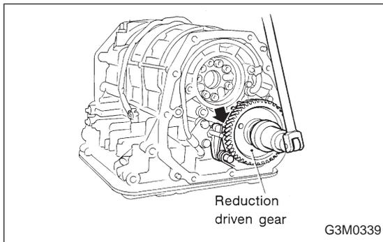
3) Install the reduction driven gear.
