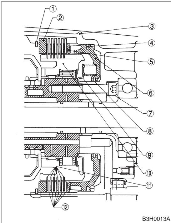
10) Installation of the low & reverse brake:
