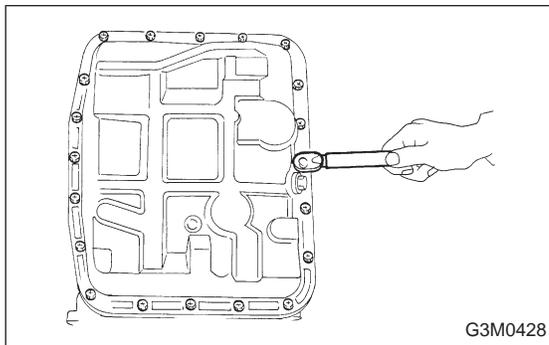
(2) With gasket inserted, secure the oil pan by tightening 20 bolts.
