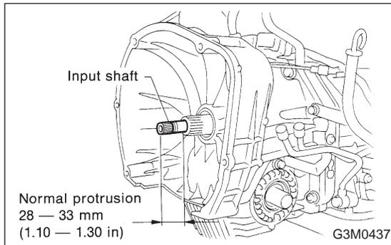
11) Insert the input shaft while turning lightly by hand.
