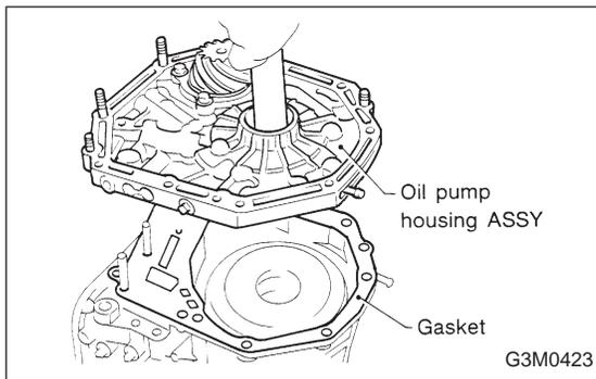
24) Install the oil pump housing assembly.
