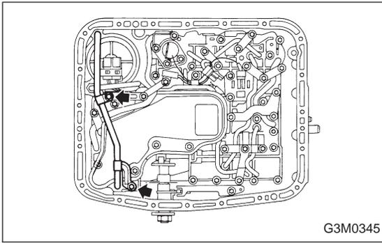
7) Remove the oil cooler outlet pipe.
