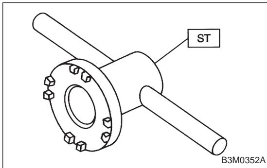
10) Using the ST, screw in the retainer until light contact is felt.
