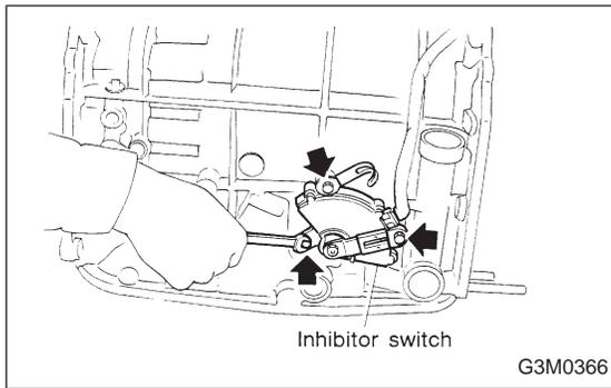
30) Remove the inhibitor switch.
