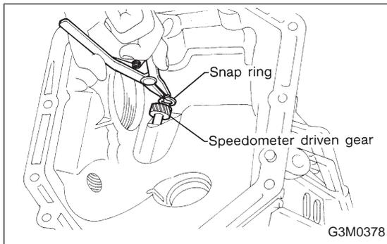
4) Install the speedometer driven gear to the speedometer shaft, and secure with a snap ring.
