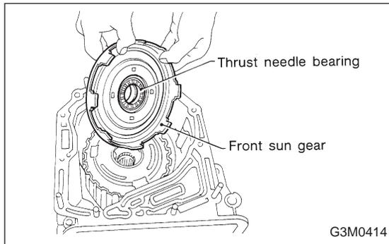
18) Install the front sun gear. Attach the thrust needle bearing to the gear, and install the gear while turning slowly.
