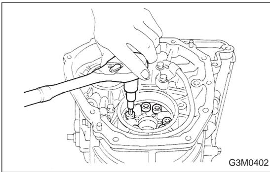
(3) Place the spring retainer on the inner race. Install the spring to the recessed portion of the piston. Then tighten eight socket head bolts from the rear side of the transmission case.
