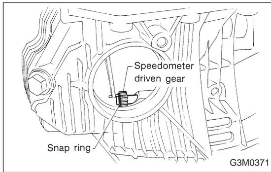
5) Remove the snap ring. Then remove the speedometer driven gear.
