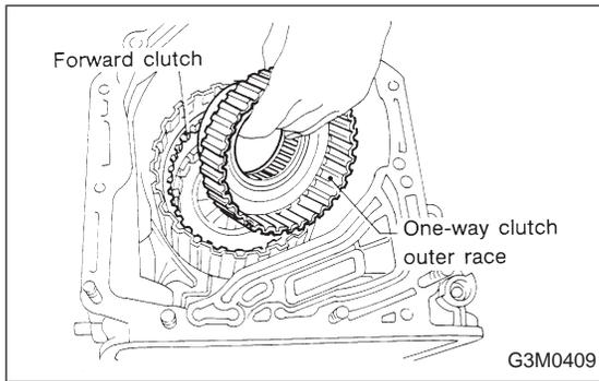
13) Install the one-way clutch outer race.
