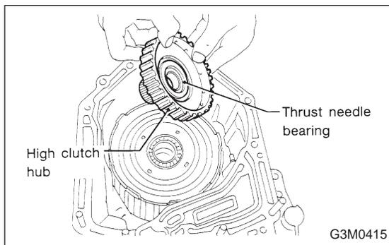
19) Install the high clutch hub. Attach the thrust needle bearing to the hub with vaseline and install the hub by correctly engaging the splines of the front planetary carrier.
