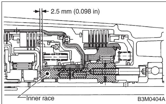
11) Install the forward clutch drum.
