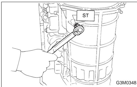
13) Loosen the brake band adjusting screw with ST, and take out the strut.
