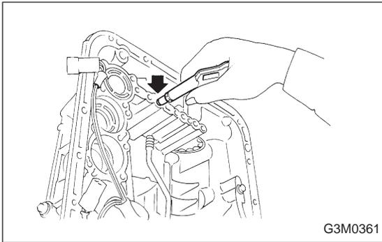
(3) Take out the low & reverse piston by applying compressed air.
