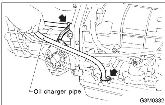
6) Install the oil charge pipe.
