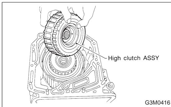
20) Install the high clutch assembly.
