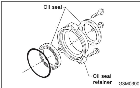
13) Install two oil seals to the oil seal retainer with ST.
