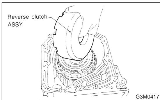
21) Install the reverse clutch assembly.
