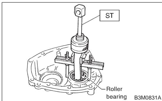
3) Take out the roller bearing inner race with ST.
