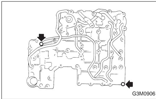
5) Temporarily assemble lower valve body to upper valve body.
