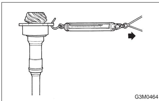
5) Measure the starting torque of the bearing.
