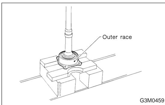
2) Using a press, separate the rear roller bearing and outer race from the shaft.
