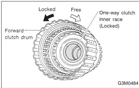
9) Install the one-way clutch (1-2) and plate, and secure with the snap ring.
