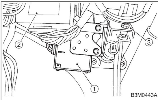
3) Remove transmission control module.
