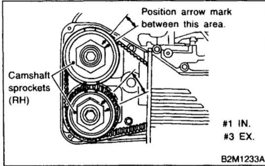
8) Ensure that #1 cylinder intake valve and #3 cylinder exhaust valve are adjusted to specifications.
