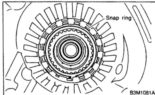
26) Take out retaining plate, drive plate, driven plate and dish plate.
