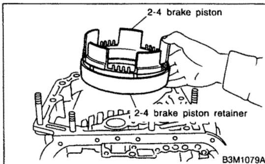
23) Separate 2-4 brake piston and piston retainer.
