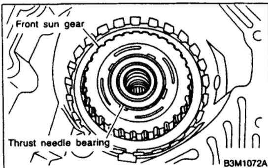
16) Remove snap ring and thrust needle bearing.
