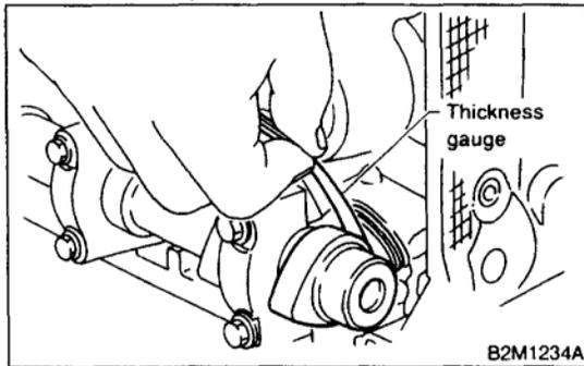
9) Turn crankshaft two complete rotations. Check again to ensure that #1 cylinder intake valve and #3 cylinder exhaust valve clearances are within specifications. If necessary, re-adjust valve clearances.
