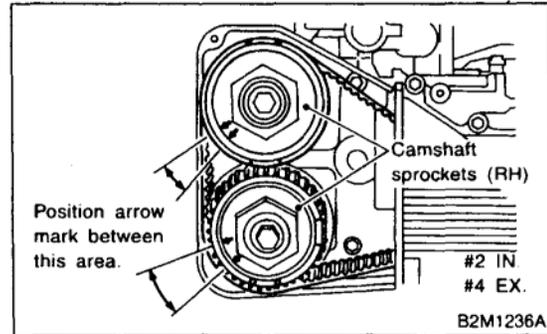
(3) Set arrow mark on camshaft sprocket to position shown in figure, and check #1 cylinder exhaust valve and #4 cylinder intake valve clearances.
