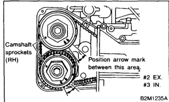
(2) Set arrow mark on camshaft sprocket to position shown in figure, and check #2 cylinder intake valve and #4 cylinder exhaust valve clearances.
