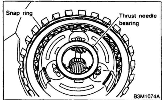
17) Take out retaining plate, drive plate and driven plate of 2-4 brake.
