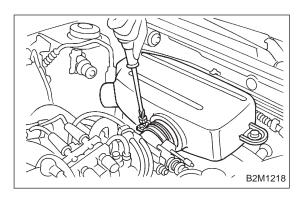
21) Install air intake chamber and connect air hoses.
