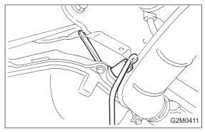
5) Remove front oxygen sensor.
