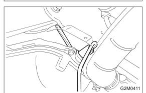
Install front oxygen sensor.
