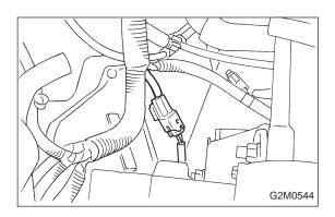
2) Disconnect connector from front oxygen sensor.
