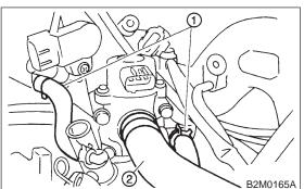
2) Disconnect engine coolant hoses (1) from idle air control solenoid valve.
