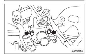
4) Remove idle air control solenoid valve from throttle body.
