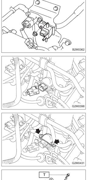
3) Remove pressure sources switching solenoid valve from bracket.
