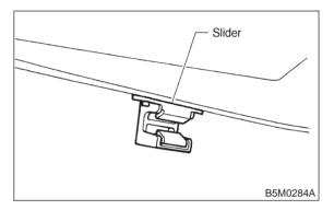
• To facilitate installation of rear bumper, insert the bumper hook into the body groove.
