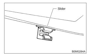
• To facilitate installation of rear bumper, insert the bumper hook into the body groove.
