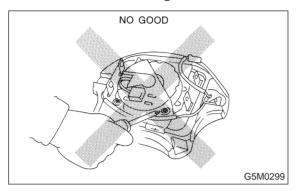
• When removing and installing the airbag module (driver, passenger and side), the operator should stand, as much as possible, on the side of the airbag module.
