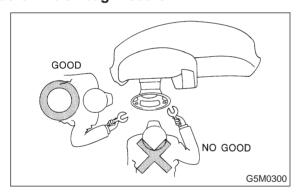
• After removal, the airbag module (driver, passenger and side) should be kept away from heat and light sources, and stored on a clean, flat surface to prevent from any damage to its lower structure.
