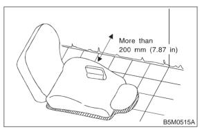
• When storing a removed airbag module (driver and passenger), be sure to place it in parallel with floor with the pad facing up. Do not place it against a wall, or place anything on the pad; otherwise, a dangerous condition may be created if the module malfunctions.
