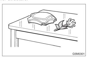
• Do not check airbag module (driver, passenger and side) continuity with airbag removed from the vehicle body.
