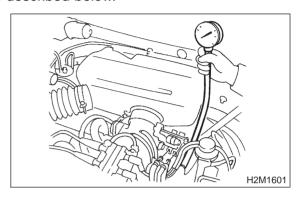
Vacuum pressure (at idling, A/C "OFF"): Less than -60.0 kPa (-450 mmHg, -17.72 inHg)
