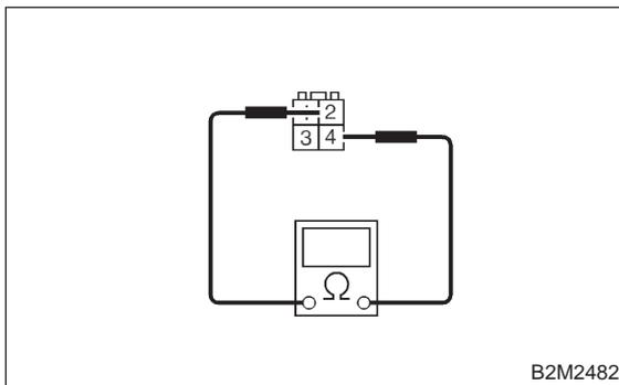
**CHECK** : *Is the resistance less than 30 Ω?*
