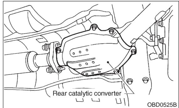
**CHECK** : Is there damage at rear face of rear catalyst?
