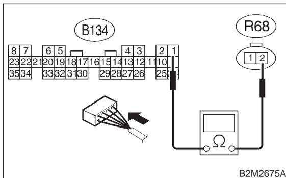
**CHECK** : Is the voltage less than 1 Ω?
