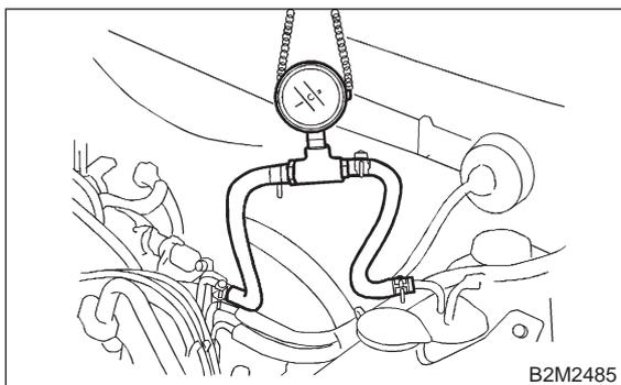
**CHECK** : *Is fuel pressure between 226 and 275 kPa (2.3 — 2.8 kg/cm<sup>2</sup>, 33 — 40 psi)?*
