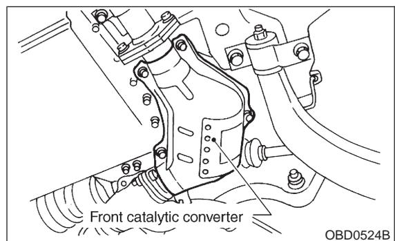
**CHECK** : Is there damage at rear face or front face of front catalyst?
