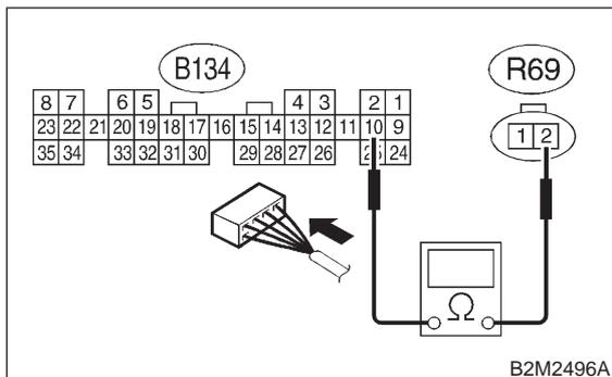
**CHECK** : Is the voltage less than 1 Ω?
