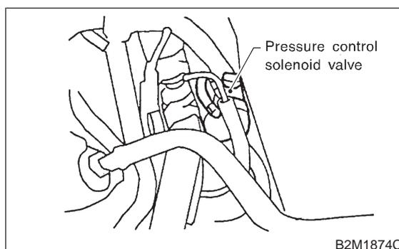
**CHECK** : *Does pressure control solenoid valve produce operating sound?*
