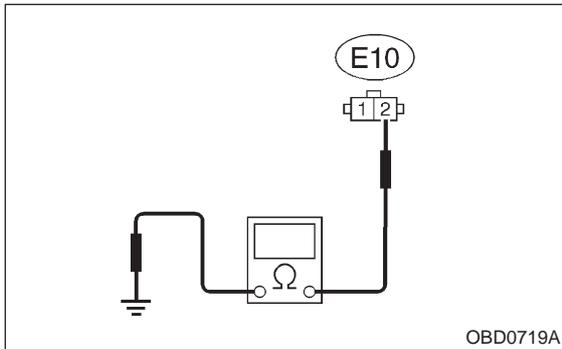
**CHECK** : *Is the resistance less than 5 Ω?*
