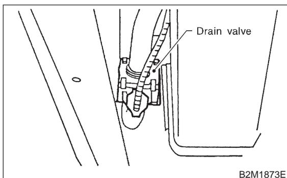
**CHECK** : *Does drain valve produce operating sound?*
