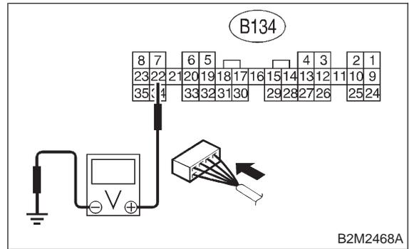
**CHECK** : **Does the voltage change more than 8 V by shaking harness and connector of ECM while monitoring the value with voltage meter?**
