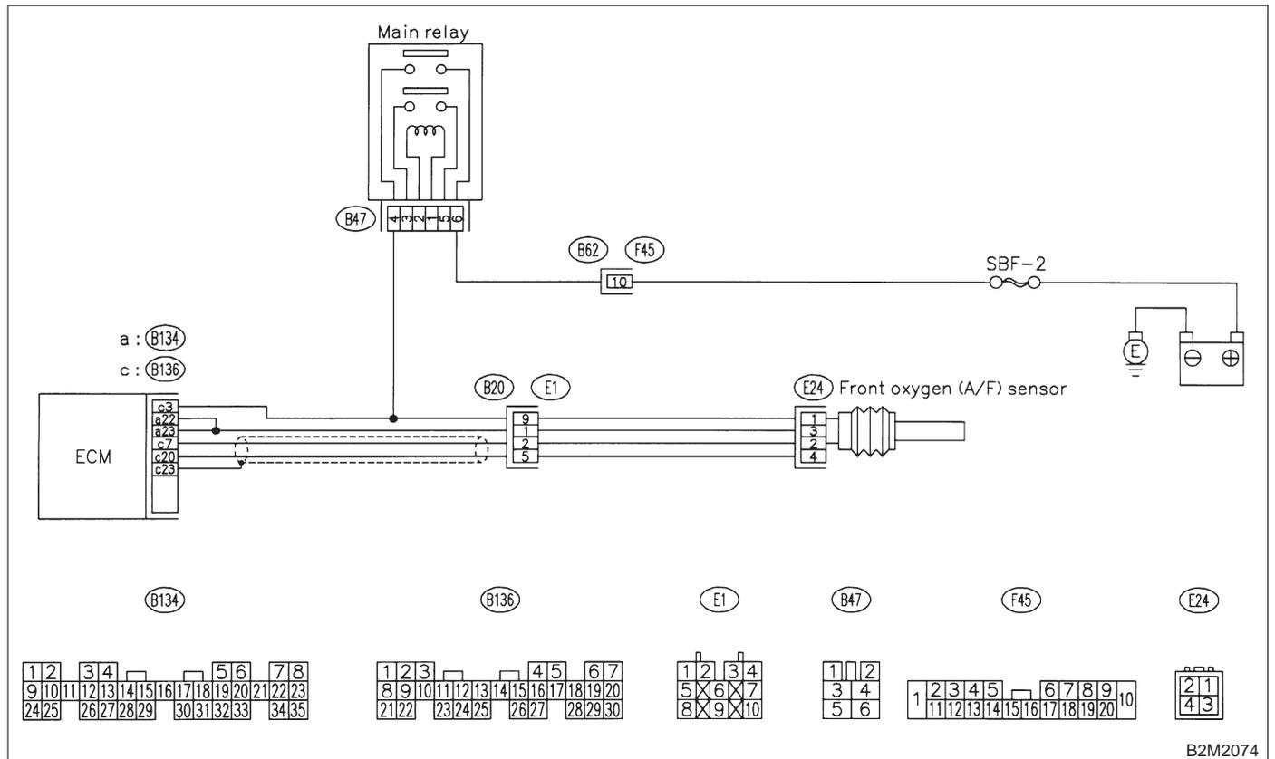
**12CA1 : CHECK HARNESS BETWEEN ECM AND FRONT OXYGEN (A/F) SENSOR CONNECTOR.**
