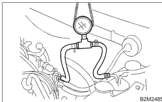
**CHECK** : *Is fuel pressure between 157 and 206 kPa (1.6 — 2.1 kg/cm<sup>2</sup>, 23 — 30 psi)?*
