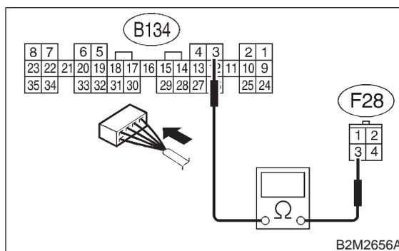
**CHECK** : Is the resistance less than 1 Ω?
