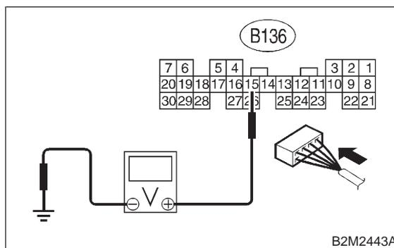
**CHECK** : *Does the voltage change more than 4.5 V by shaking harness and connector of ECM while monitoring the value with voltage meter?*
