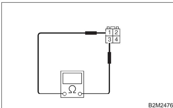
**CHECK** : *Is the resistance less than 5 Ω?*
