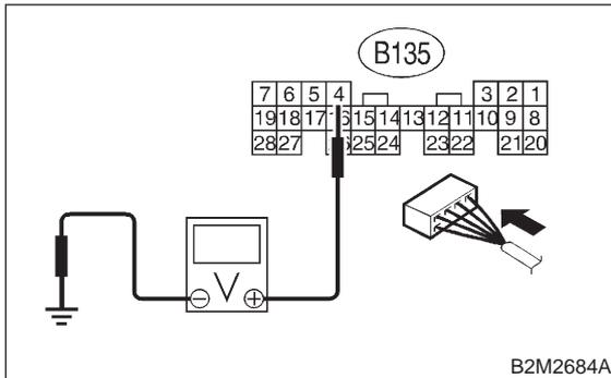
**CHECK** : Does the voltage change from 1 V to 4 V while monitoring the value with voltage meter?
