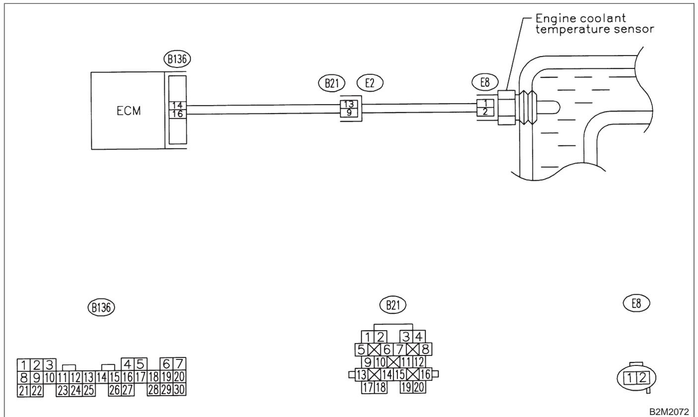
**12I1 : CONNECT SUBARU SELECT MONITOR OR THE OBD-II GENERAL SCAN TOOL, AND READ DATA.**
