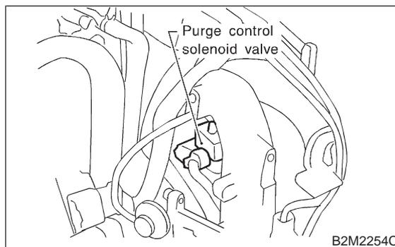
**CHECK** : *Does purge control solenoid valve produce operating sound?*
