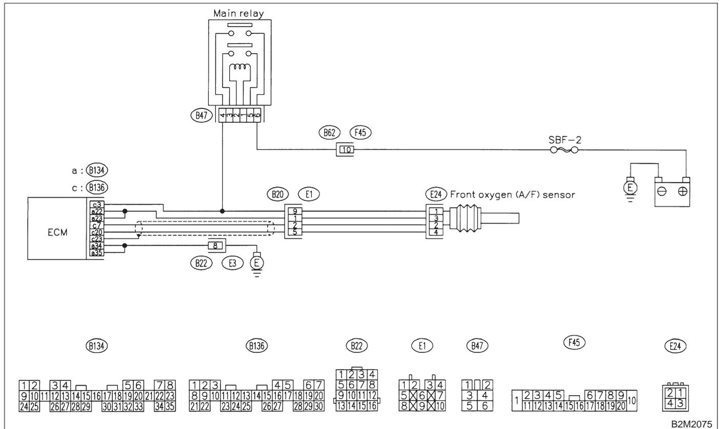
**12CF1 : CHECK HARNESS BETWEEN ECM AND FRONT OXYGEN (A/F) SENSOR CONNECTOR.**
