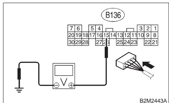
**CHECK** : *Does the voltage change more than 4.5 V by shaking harness and connector of ECM while monitoring the value with voltage meter?*
