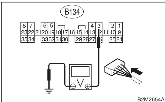
**CHECK** : Does voltage change between 0 and 10 volts?
