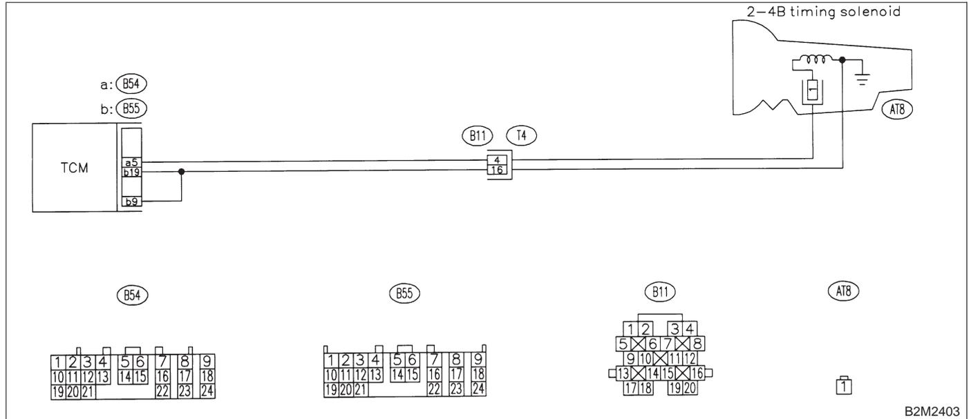
**12CV1 : CHECK DTC P1704 ON DISPLAY.**
