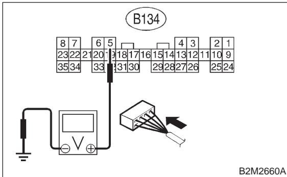
**CHECK** : **Does the voltage change more than 10 V by shaking harness and connector of ECM while monitoring the value with voltage meter?**
