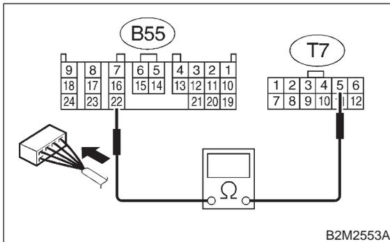
**CHECK** : *Is the resistance less than 1  $\Omega$ ?*
