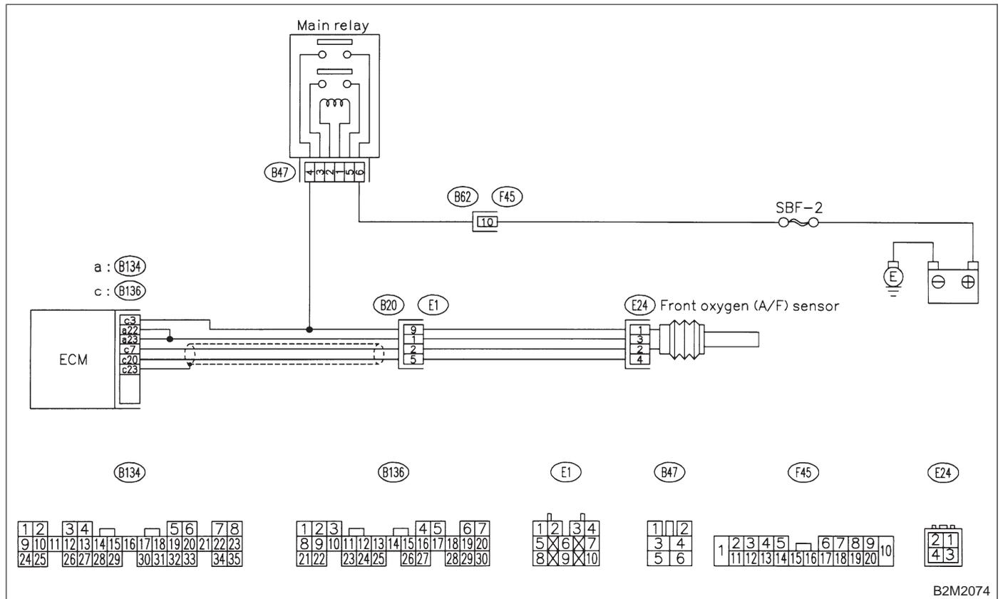
**12CB1 : CHECK HARNESS BETWEEN ECM AND FRONT OXYGEN (A/F) SENSOR CONNECTOR.**
