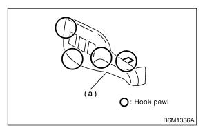
2) Remove main switch by pushing it outward.
