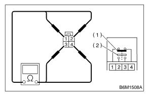
Check continuity brake switch (1) and stop light switch (2) between terminals.
