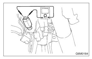
Check continuity between clutch switch terminals.
