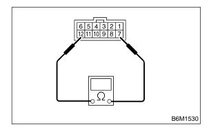
Check continuity between inhibitor switch terminals.
